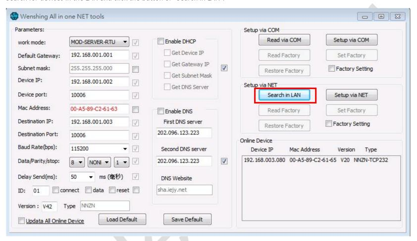
3. After searching for the device and the IP address of the device will be displayed below.
