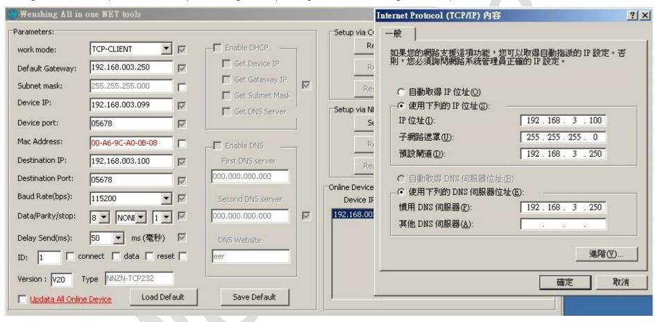
10. Test on the communication, PC execute "TCP Server" software and set the appropriate port. Send the AT command to test the communication is correct or not.
