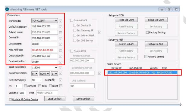
6. Modify the setting parameter on internet. Find the suitable setting on the left and correct it. Click "Setup via NET" to modify it. (Device Port > Destination Port cannot set to 5978. This Port is for online update only.)
