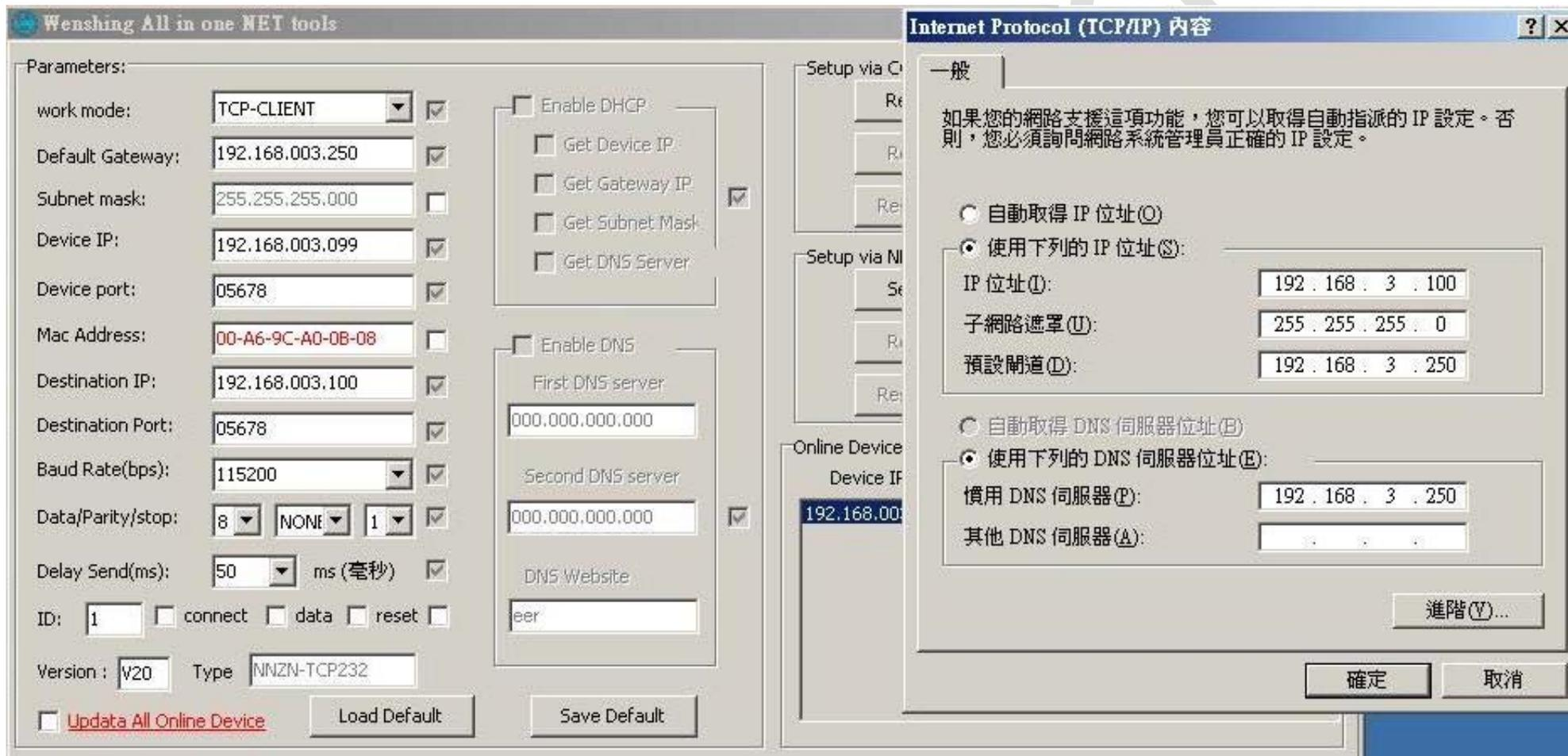
2. Test on the communication, PC execute "TCP Server" software and set the appropriate port. Send the AT command to test the communication is correct or not. (cannot use Port 5978).
